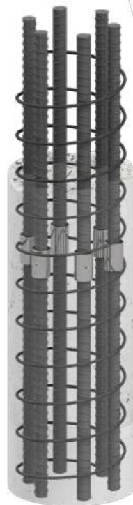
**Circular Column Rebar Connections**
